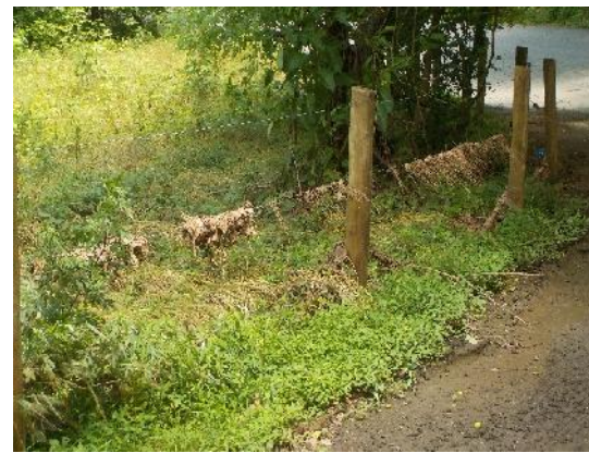
Figure 6: Debris @ Milton fence showing flood water levels
