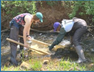
Volunteer monitors follow strict protocols to collect benthic macroinvertebrates with a net.
